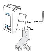
Align the wall bracket with the three pre-drilled holes on the wallboard. Screw the three supplied screws (5600-HWWB-00) into the wallboard. Avoid over-tightening as this can damage the wallboard.
