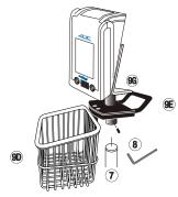
Attach metal basket to platform using two 3 mm hex screws. Tighten with small hex key provided.
