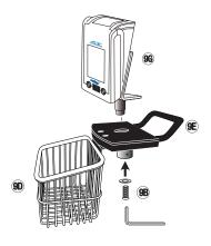
Slide stainless steel inner pole inside outer pole with open end up. Make sure shock absorbing spring is inside the outer pole and tighten.
