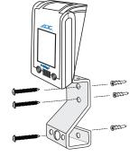
4. Next, attach the basket to the wall bracket. Align the basket screw holes with the bracket screw holes and insert the two supplied basket bolts (9005MBAS-S-00) through these openings. Tighten the bolts firmly to secure the basket in place.
