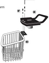
Attach the e-sphyg<sup>3</sup> to the mounting bracket using short 2 mm hex screws and washers as shown.
