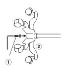
6. Place assembly consisting of the e-sphyg<sup>3</sup>, cuff storage basket and platform on top of stainless steel inner pole, making sure the pole goes completely inside collar. Use tightening device and small hex key as shown.
