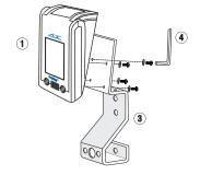
Attach wall bracket to wall. For optimum viewing, it is suggested that you measure 60" from the floor to the top of the wall mounting bracket (or add just as needed). Once positioned to desired height, mark screw positions on the wall making sure bracket is level. Screw three supplied screws firmly into a stud, or use the three supplied anchors to secure to the wall.
