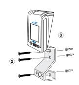
3. After the unit and wall bracket have been attached to the wall, position the basket onto the bracket and screw the two basket screws through the basket openings and tighten.
