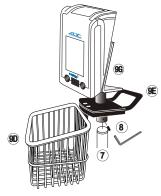
Slide stainless steel inner pole inside outer pole with open end up. Make sure shock absorbing spring is inside the outer pole and tighten.
