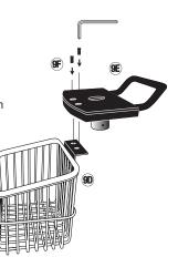
Attach the e-sphyg<sup>3</sup> to the mounting bracket using short 2 mm hex screws and washers as shown. Tighten with small hex key.
