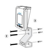
After the unit and wall bracket have been attached to the wall, position the basket onto the bracket and screw the two basket screws through the basket openings and tighten.
