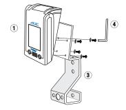
2. Attach wall bracket to wall. For optimum viewing, it is suggested that you measure 60" from the floor to the top of the wall mounting bracket (or add just as needed). Once positioned to desired height, mark screw positions on the wall making sure bracket is level. Screw three supplied screws firmly into a stud, or use the three supplied anchors to secure to the wall.
