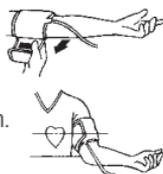
**Important!** The small white  $\Phi$  (Artery Mark) on the cuff must lie exactly over the artery which runs down the inner side of the arm.
